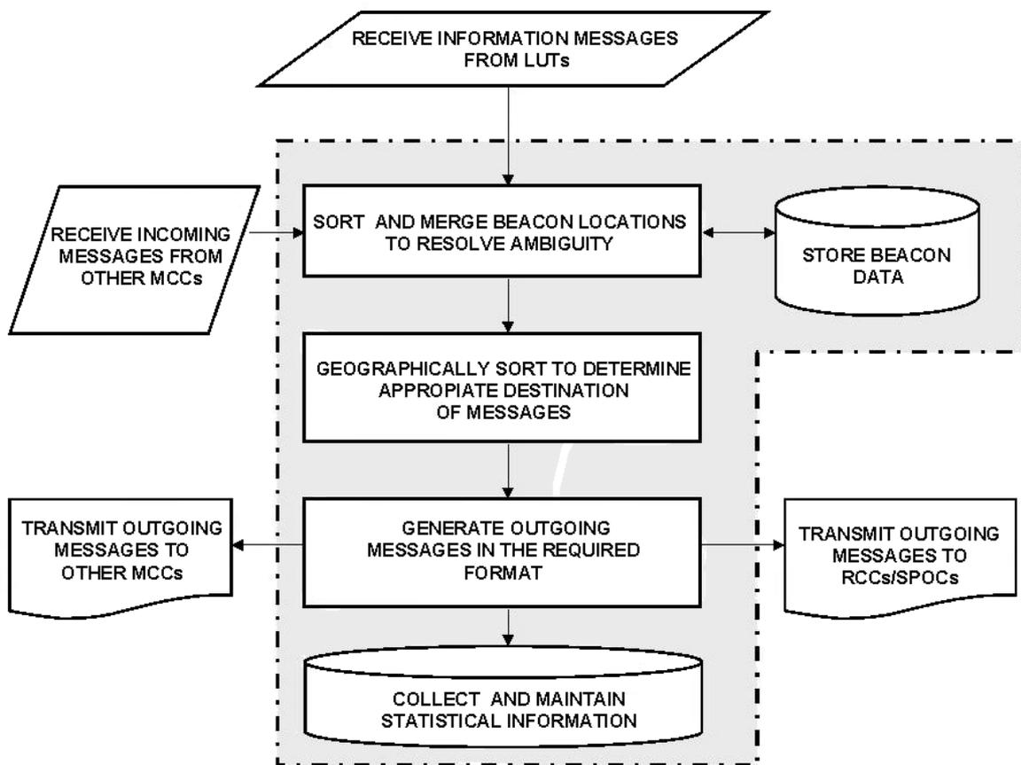
**Figure 4.2: Functional Diagram of Alert Data Processing by MCCs**
