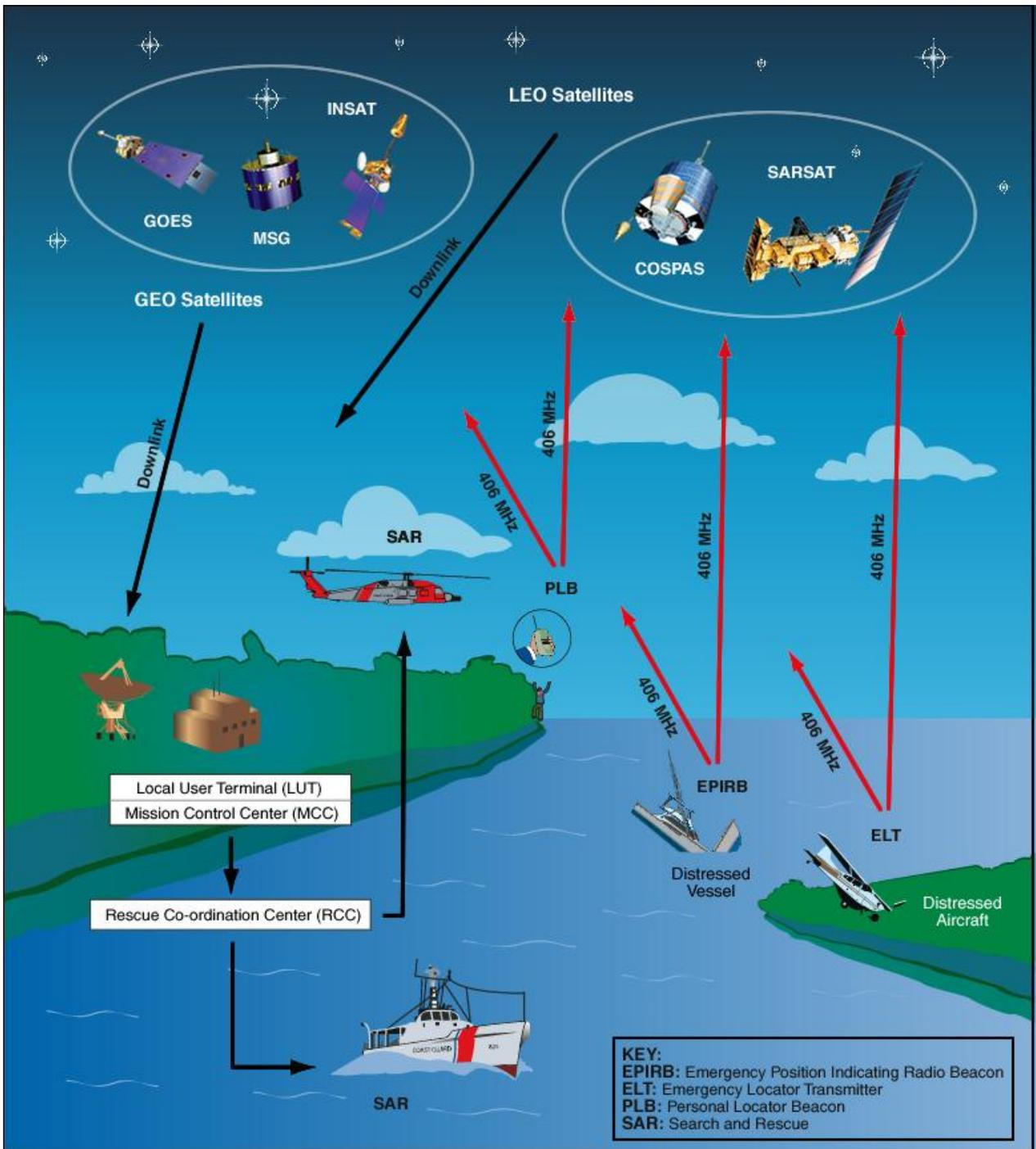
**Figure 2.1 : Basic Concept of the Cospas-Sarsat System**
