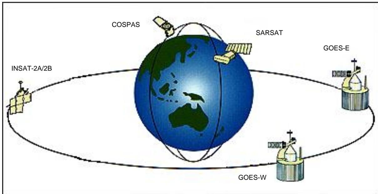
**Figure 3.2: Combined LEOSAR - GEOSAR Operations**
